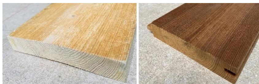
Figure 11: (left) Raw wood of Scots pine, (right) Thermal-D wood.
