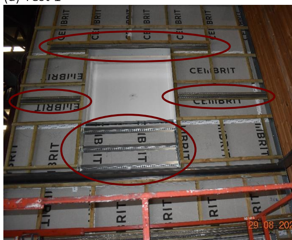
Figure 20: Distribution of the ventilation cavity fire stops in test 1 and test 10
