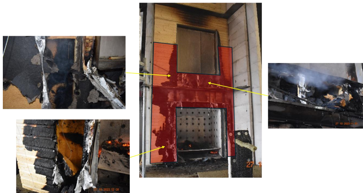
Figure 26: Areas affected by smoldering insulation (Test 3)
