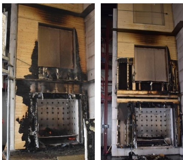
Figure 35: Charred areas after test (left) and dismantled areas, where smoldering was observed (right) in Test 3
