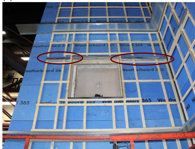
Figure 20: Distribution of the ventilation cavity fire stops in test 1 and test 10
