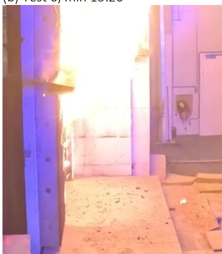
Figure 31: Formation of burning parts at the base of the façade rig
